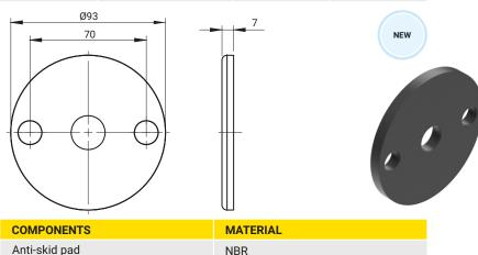
\* The anti-skid pad 4.519.100 works with the oscillating feet 4.519
