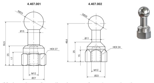
Ball studs mounted on power rails, power cables, or other components of power equipment are used to attach the phase terminals of the earth electrode to the ball studs.
