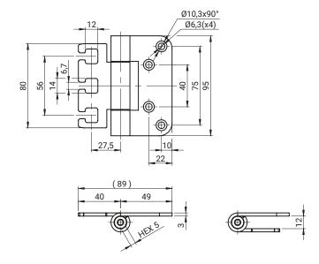
The hinge with 3D adjustment vertically and horizontally +/- 3.0 mm works with the cassette (3.ST500.001 or 3.ST500.002) with page 3A-76 mounted to the frame.
