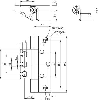
The hinge with 3D adjustment vertically and horizontally +/- 3.0 mm works with the cassette (3.ST500.001 or 3.ST500.002) with page 3A-76 mounted to the frame.
