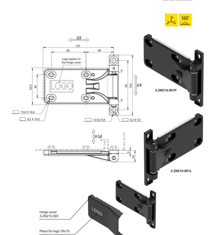
A - axis of the hinge with plastic sleeves.
