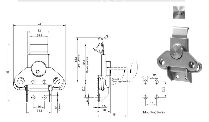
Latch opens by lifting the knob and turning counterclockwise.
