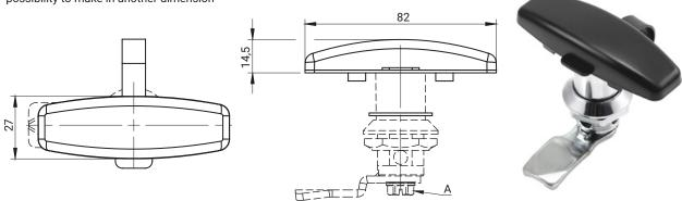
In order to mount the dust cover on the T-handle lock, remove the knob from the lock body by unscrewing the screw (A), then pass the cover through the lock pivot. In order to disassemble repeat in reverse order.
