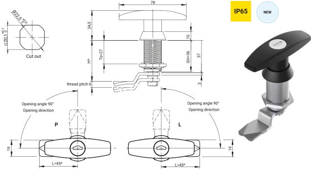
Lock in closed position - to open, unlock the cylinder and then turn the handle 180 ° to the right
