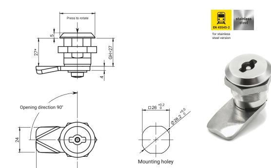
Lock with protection from undesirable opening without specific key. Rotation of locking cam is possible after pushing pin by key. Key removal possible only in locking positon of the lock. Lock works with key 2.KL-D5.001 (pg. 2A-130, 133, 136).
