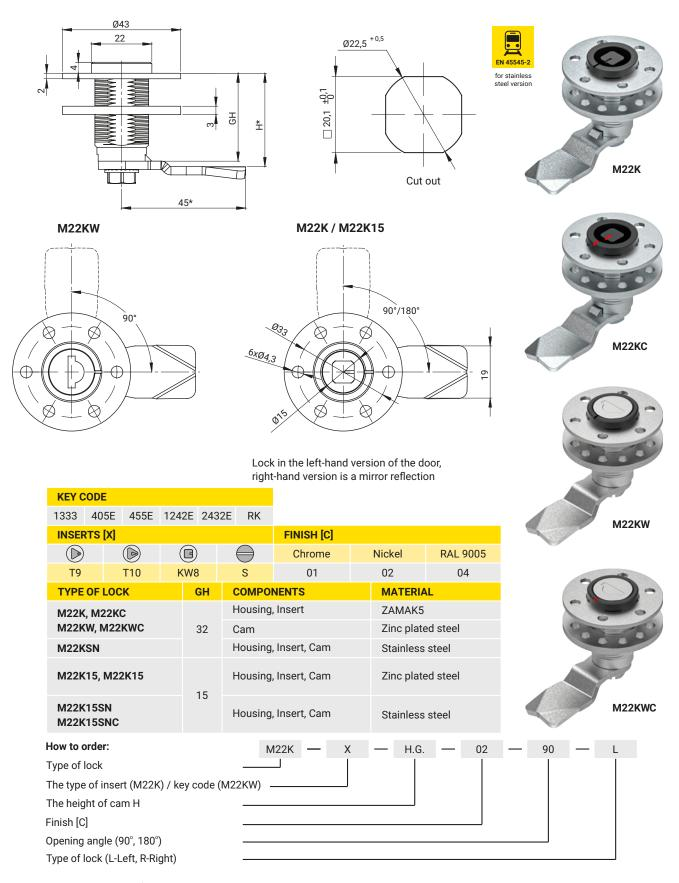
Lock at the height of GH=15mm is available only in a version with shaped insert
