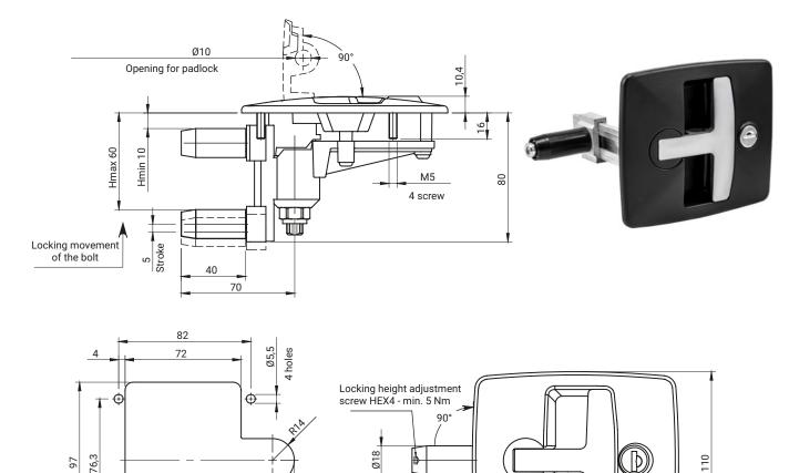
Sealing of lockable doors by folding the lock handle into the lock body.
