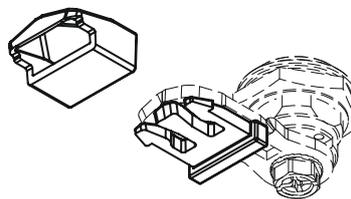
3. Holding the clip and the cam slide the cap on completely
