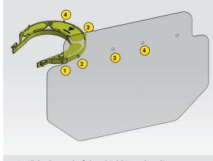
Slide the end of the shield into the clip 1
