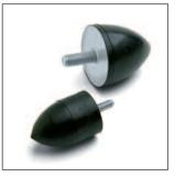
NR Rubber compound 65°±5° shore A. Zinc plated steel stud. Used as shock-absorbers, feet and stroke end. Cp: Max. compression load(Kg).
